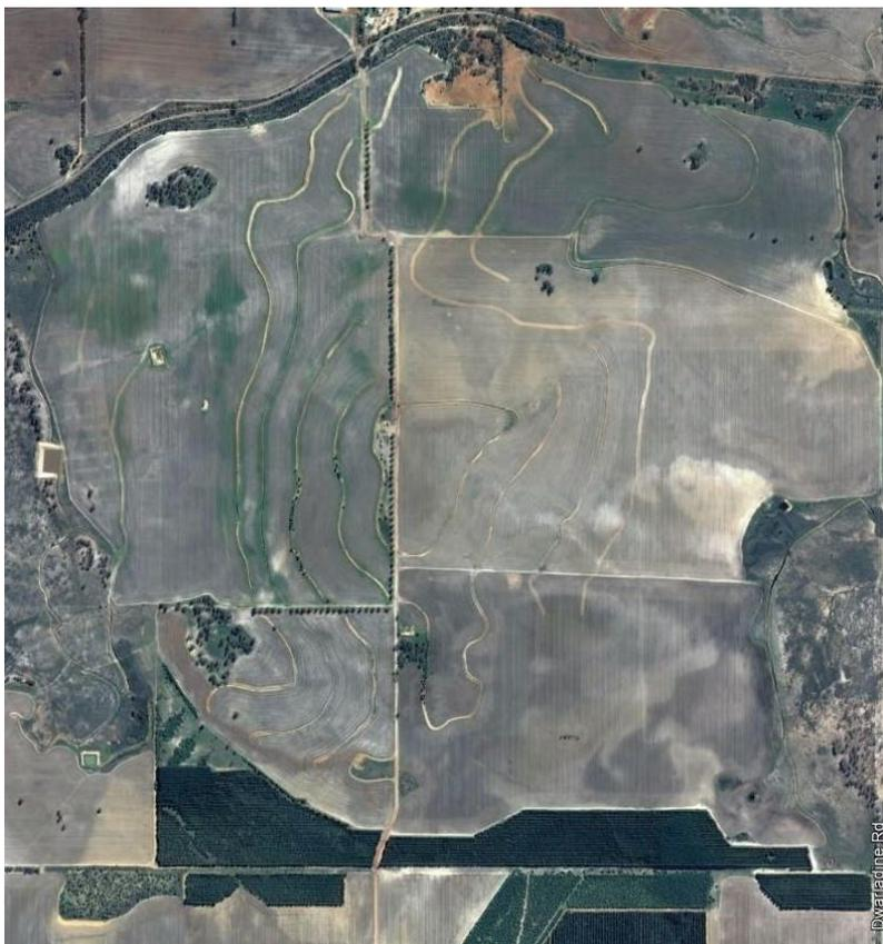
Figure 8: Showing image of Interceptor Banks installed on Darrell's farm during the 90's. Some of these banks are now filled in and replaced with Interceptor Barriers allowing easy working of paddocks.
